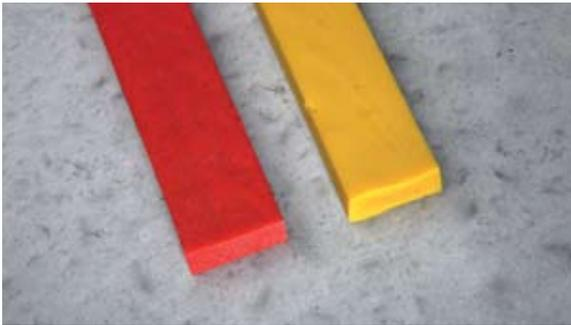
This active joint sealing system swells in contact with any water. The properties of this material enable it to swell into small cracks or gaps. SikaSwell®-A is based on acrylic resins.
