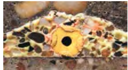
Cross-section depicting two separate injections: The first injection consisted of the yellow material; the orange material was delivered via a second injection.
