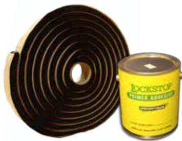
**Lockstop** is a single component and self-sealing mastic waterstop which bonds to concrete to prevent moisture from penetrating nonmoving joints. Lockstop must be used in conjunction with **Lockstop Primer Adhesive** to create a watertight bond.
