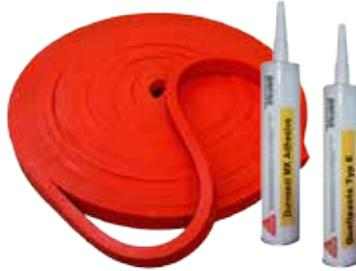
**SikaSwell®-A** (formerly Duroseal Gasket) is a water-swelling acrylate-ester that expands upon contact with water to form a compression seal in nonmoving concrete joints. SikaSwell®-A is available in three sizes and is adhered to varying substrates with **Sika® MK Adhesive** or **Quellpaste Type E**.
