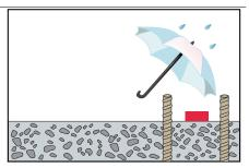
During concreting, compact the concrete well around SikaSwell®-A profile. This will ensure that a dense concrete, without any honeycombs or voids, is produced.
