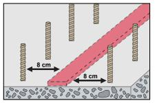
Apply SikaBond® Construction Adhesive or SikaSwell® S-2 to the prepared surface (see Product Data Sheets for specific material details).
