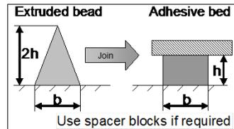
Figure 1: Recommended Bead Configuration
