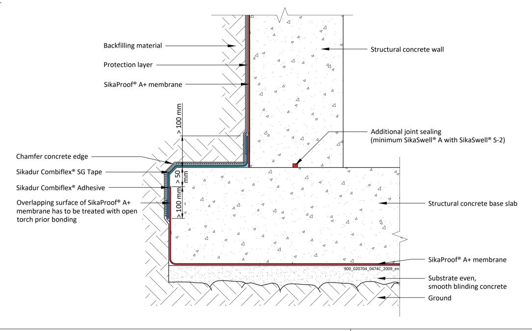
SikaProof® A+ TRANSITION BASE SLAB TO WALL WITH TOE With Sikadur-Combiflex® SG System 900\_020704\_0474C\_2009\_en September 2020
