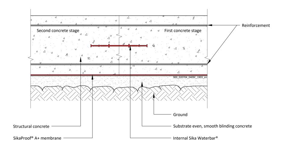
SikaProof® A+ CONSTRUCTION JOINT With internal Sika Waterbar® 900\_020704\_0409C\_2009\_en September 2020
