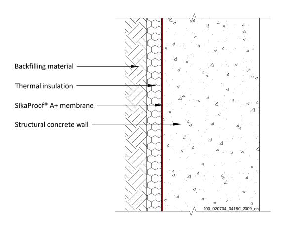
SikaProof® A+ GENERAL MEMBRANE LAYOUT With thermal insulation 900\_020704\_0418C\_2009\_en September 2020
