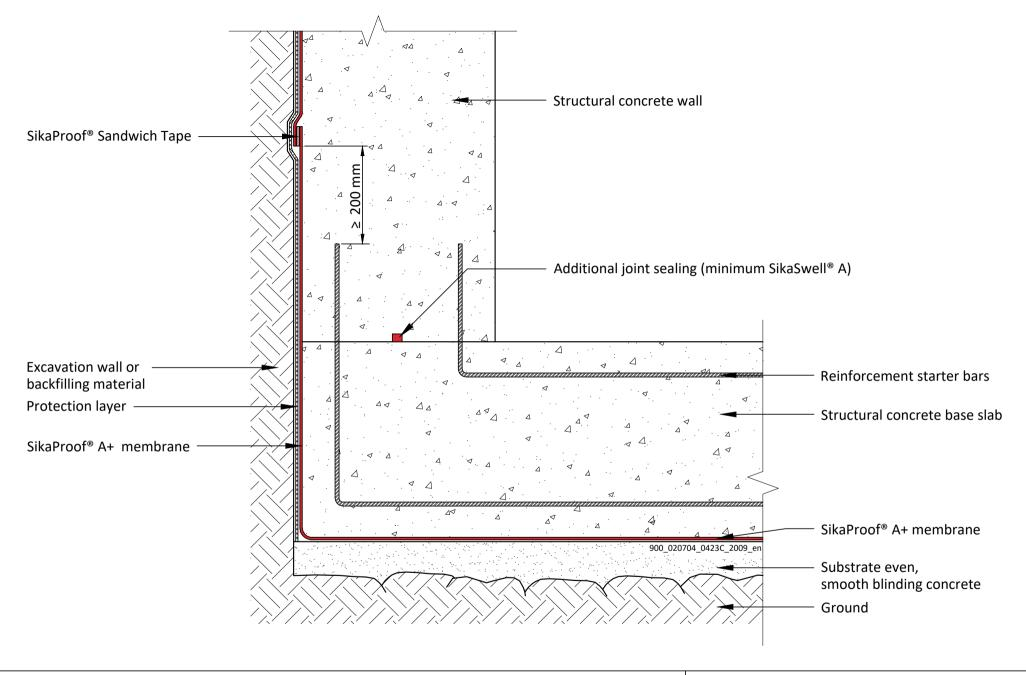
SikaProof® A+ TRANSITION BASE SLAB TO WALL With SikaProof® Sandwich Tape 900\_020704\_0423C\_2009\_en September 2020
