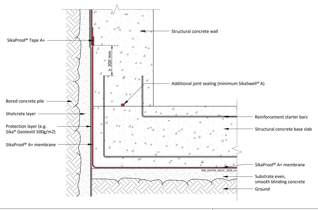
SikaProof® A+ TRANSITION BASE SLAB TO WALL Shotcrete Blinding with SikaProof® Tape A+ 900\_020704\_0652C\_2009\_en September 2020
