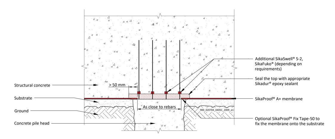
SikaProof® A+ PILE HEAD DETAIL Without levelling 900\_020704\_0405C\_2009\_en September 2020
