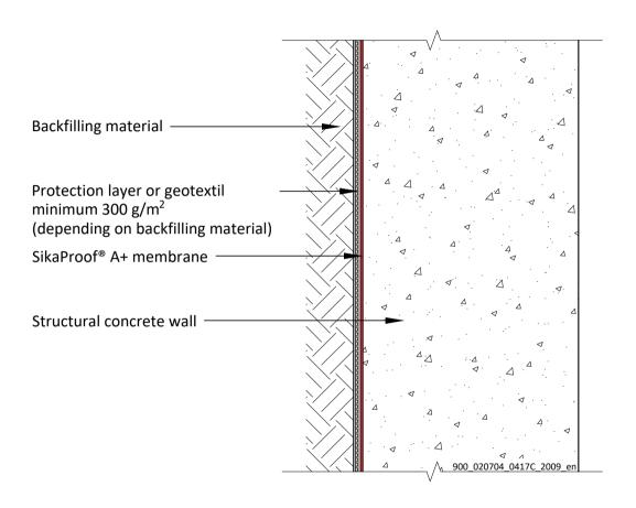
SikaProof® A+ GENERAL MEMBRANE LAYOUT With protection layer or geotextil 900\_020704\_0417C\_2009\_en September 2020
