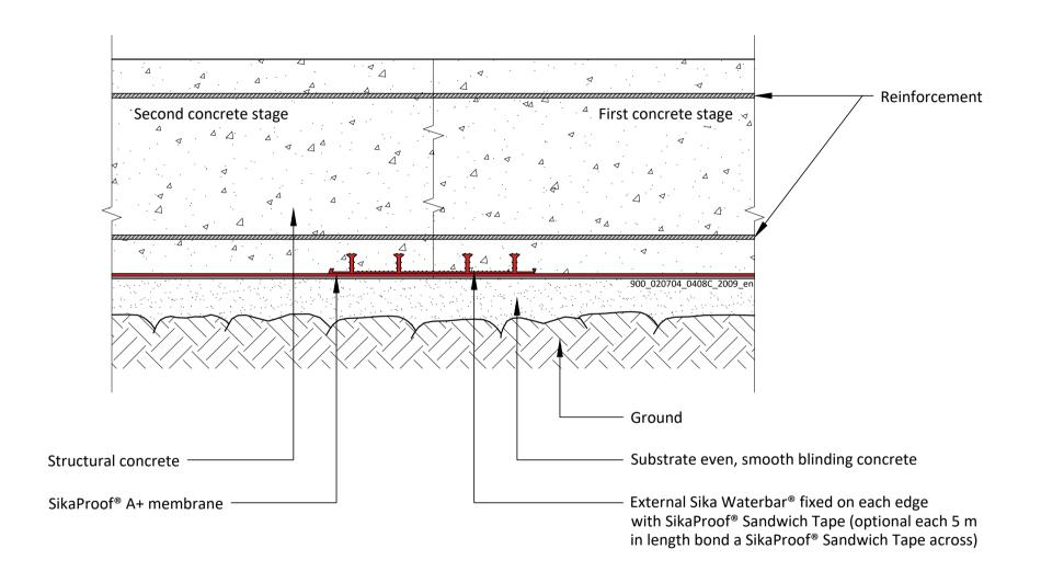
SikaProof® A+ CONSTRUCTION JOINT With external Sika Waterbar® 900\_020704\_0408C\_2009\_en September 2020
