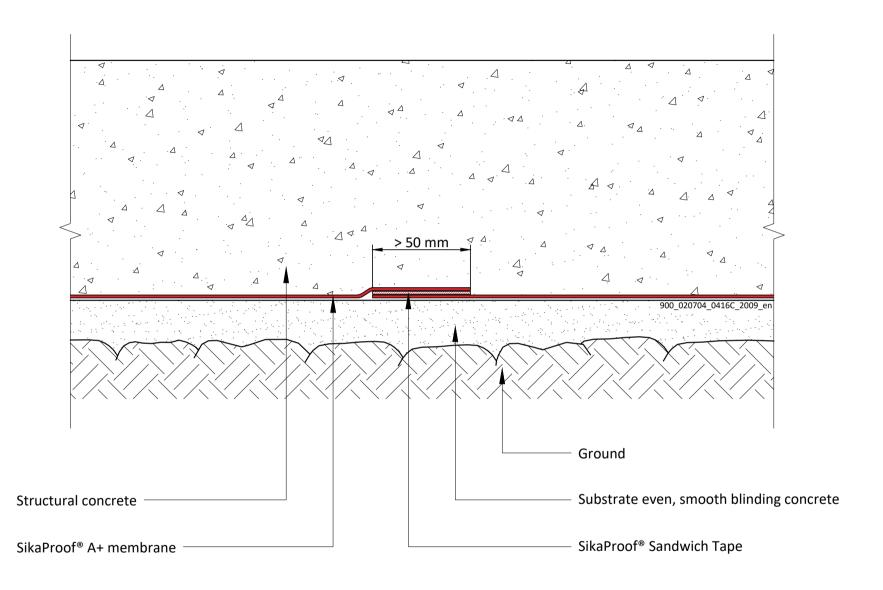
SikaProof® A+ GENERAL OVERLAP JOINT With SikaProof® Sandwich Tape 900\_020704\_0416C\_2009\_en September 2020
