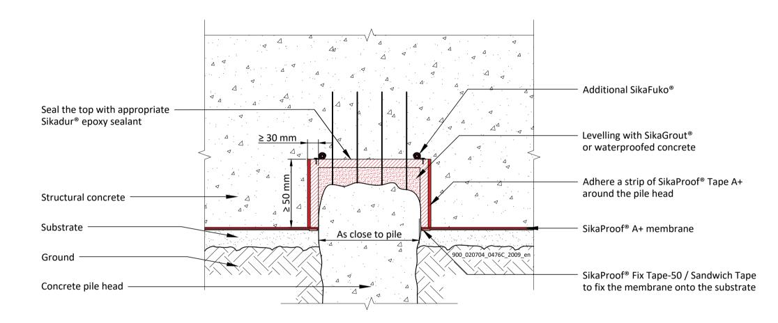
SikaProof® A+ PILE HEAD DETAIL FOR TENSION PILES With levelling and SikaProof® Tape A+ 900\_020704\_0476C\_2009\_en September 2020
