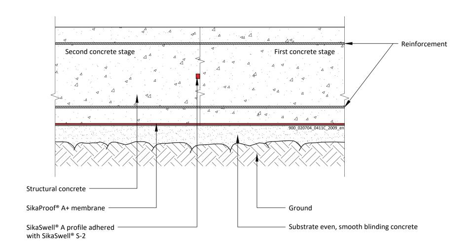
SikaProof® A+ CONSTRUCTION JOINT With SikaSwell® A / S-2 900\_020704\_0411C\_2009\_en September 2020
