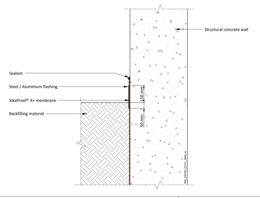
SikaProof® A+ TERMINATION AT CONCRETE WALL With sealant and steel or aluminium flashing 900\_020704\_0721C\_2009\_en September 2020
