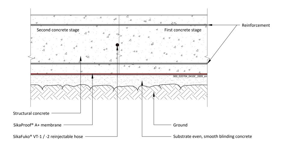
SikaProof® A+ CONSTRUCTION JOINT With SikaFuko® injection hose 900\_020704\_0410C\_2009\_en September 2020
