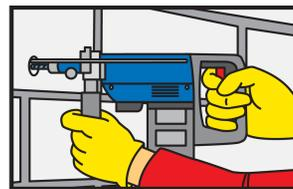
Drilling of hole with an electric drill to the diameter and depth required. Drill hole diameter must be in accordance with anchor size.
