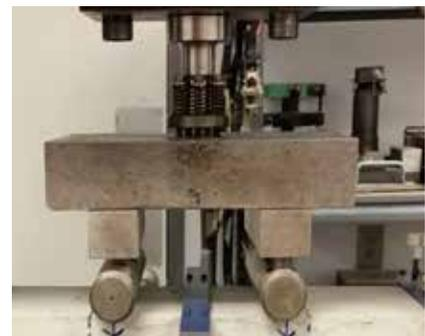
Beam test: ASTM C1609
