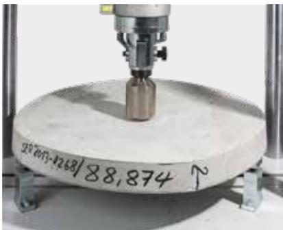
Round panel test: ASTM C1550
