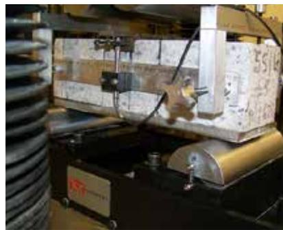
Beam test: ASTM C1399
