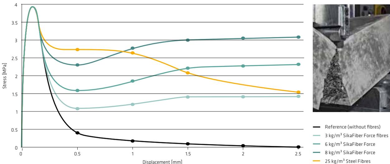
With this graphic you can see that the steel fibre-reinforced concrete exhibits the higher elastic modulus and the largest stress capacity after the first crack. Due to the shorter steel fibre length (35 mm) this stress level decreases with increasing
