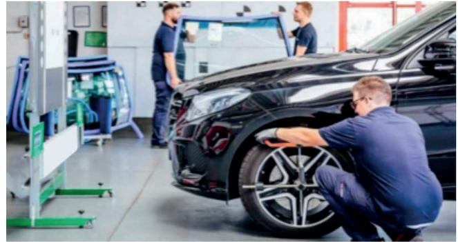
Therefore, after the replacement and prior the vehicle being handed over to the driver, a recalibration of ADAS is needed to secure road safety. Independent of the climate or the location that the replacement of the windshield is executed. The installation and calibration must be precise and follow a defined process.
