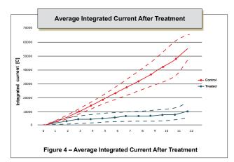
Figure 4 taken from the test report indicates "the corrosion rate in the treated slabs was significantly lowered. This can be seen by the slope of the curves in figure 4"
