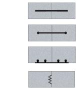
**Flat Ribbed profiles** are preferred for non-moving joints and provide the best sealing characteristics.
