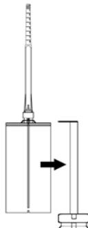
**Note:** The SAF-Q2 nozzle is in two sections. One section contains the mixing elements and the other section is an extension piece. Connect the extension piece to the mixing section by pushing the two sections firmly together until a positive engagement is felt.
