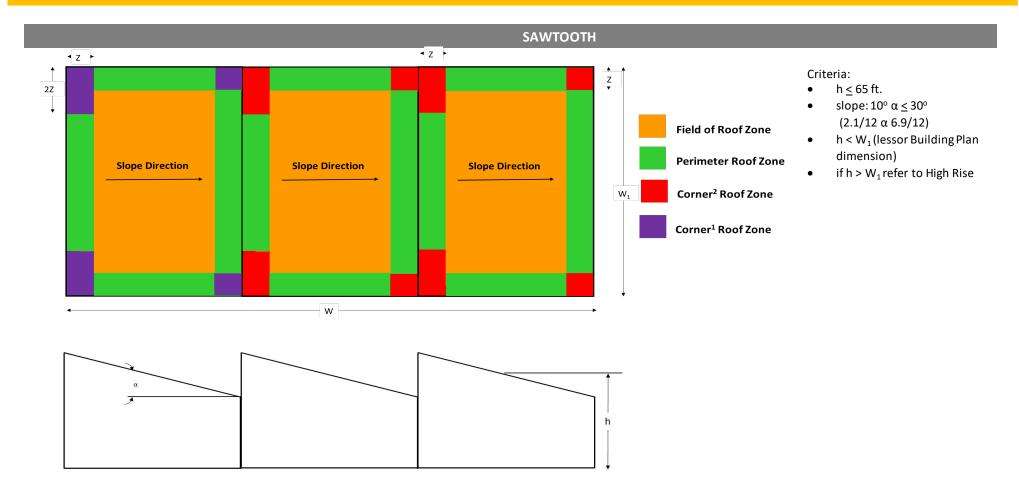
Calculation: Z = Lessor of: 40 % of the Roof Height (h) or 10 % of the lessor Building Plan (NOT ROOF) dimension (W<sub>1</sub>), but not less than 4 % of W<sub>1</sub>
