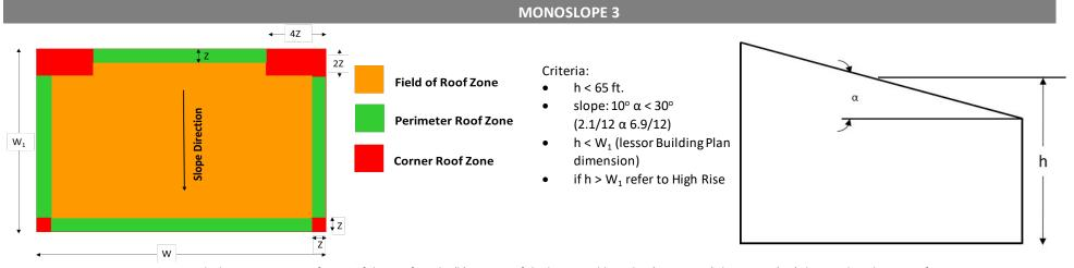
Calculation: Z = Lessor of: 40 % of the Roof Height (h) or 10 % of the lessor Building Plan (NOT ROOF) dimension (W<sub>1</sub>), but not less than 4 % of W<sub>1</sub>
