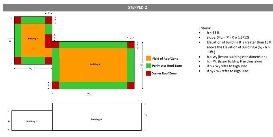
Note: Z is to be calculated separetly for Building A and Building B.
