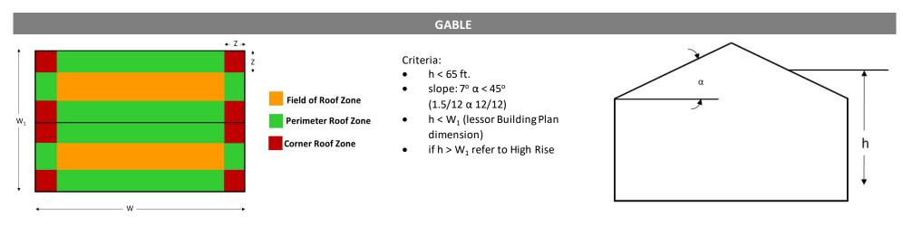
Calculation: Z = Lessor of: 40 % of the Roof Height (h) or 10 % of the lessor Building Plan (NOT ROOF) dimension (W<sub>1</sub>), but not less than
