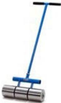
After the membrane is laid into the adhesive it should be immediately broomed, followed immediately by rolling with a 45 kg (100 pounds) or heavier, linoleum roller. Brooming alone is not sufficient to ensure the membrane is securely and evenly adhered. On steep slopes the roller will need to be tied off and lowered down from above.
