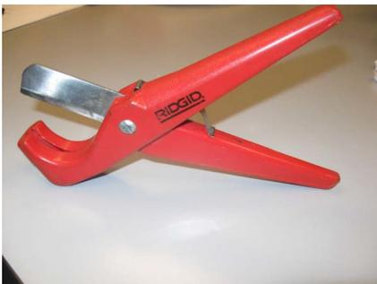
Cutting the ribs can be done with a fine-toothed saw (CAUTION: Do not cut the membrane) or with a rigid pipe cutting tool as shown here.
