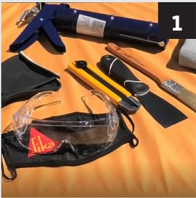
**1** Wear necessary personal protective equipment for application: safety gloves, protection mask and safety glasses.
