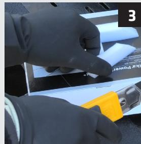
**3** Cut a **Sika® PowerClean Aid** pad to the size required for the application with a snap-off utility knife.
