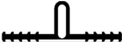
**Tear Web** - Use Where Large Movements Are Expected. Tear Web Keeps Concrete Out Of The Bulb During Concrete Placement. Upon Joint Movement, The Thin Tear Web Ruptures Allowing Substantial Mechanical Deformation Of Center Bulb Without Stressing The Material.
