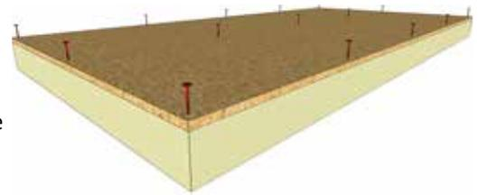
**Multi-Layer Insulation Systems** - Rmax recommends two layers of insulation whenever the total insulation requirement exceeds 3.0" to reduce thermal bridging, moisture migration and system movement. Multi-Layer systems utilize Multi-Max® FA-3 or Ultra-Max® as the bottom layer prior to installing the Nailable Base-3. Joints should be offset between the insulation layers as well as between the insulation and cover board.
