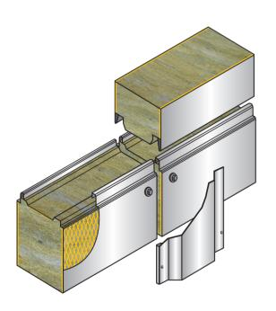
Metal faced panels with foam or mineral wool core are widely used in insulated building panels.
