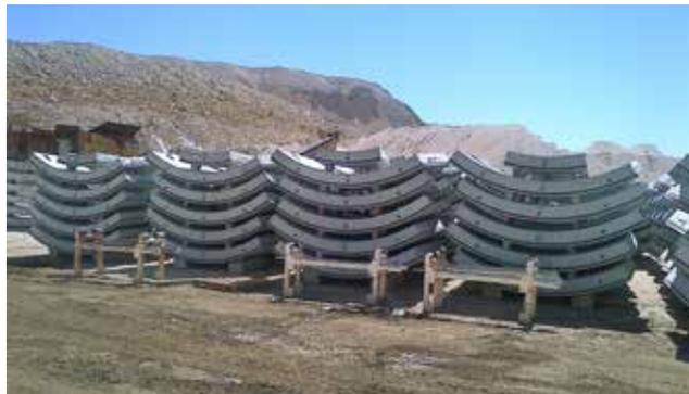
In the San Francisco Central Subway Project, SikaFiber® synthetic micro-fibres were used at a dosage of 1.2 kg/m<sup>3</sup> of concrete to prevent explosive spalling of concrete in the event of fire in the tunnel.
