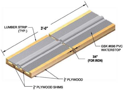
Figure 4: Example plywood welding table
