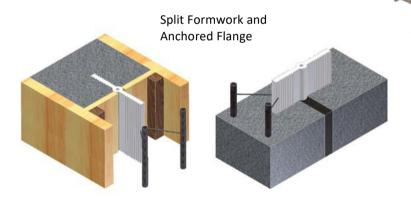
Waterstop should be aligned with the center of the joint. Size and style of the waterstop determine permissible variation from the centerline. Contact sika for specific guidelines.
