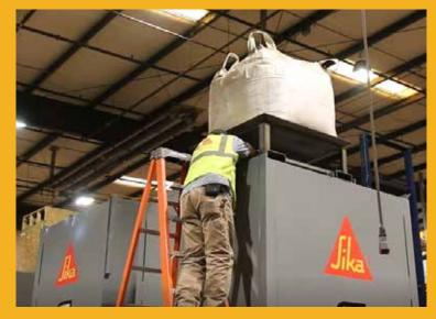
We put safety first by designing the CHROMIX-It 404° Series so that the supersacks can be untied while the cradle sits firmly on top of the machine.
