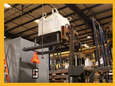
Loading totes of color is easy with the CHROMIX-It® 404 MER Granular Color Dispenser. You simply place the tote onto the supplied cradle (left above), and then place he cradle atop the machine, where it slides in between metal guide rails (right above).
