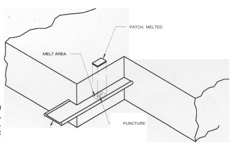
size to extend beyond the damaged area on all edges by approximately 12 mm (1/2 in). The area surrounding the damage will need to be heated until a layer (approximately 3 mm [1/16 in] thick) of melted PVC material develops. This requires the use of a thermostatically controlled, Teflon coated, heating iron.
