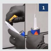
Cut the nozzle of the **Sikaflex®-291** to the desired joint width and puncture the aluminum membrane of the cartridge.
