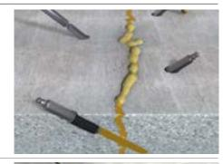
Leaking Expansion Joints (movement) and Construction / Daywork Joints (non-moving)
