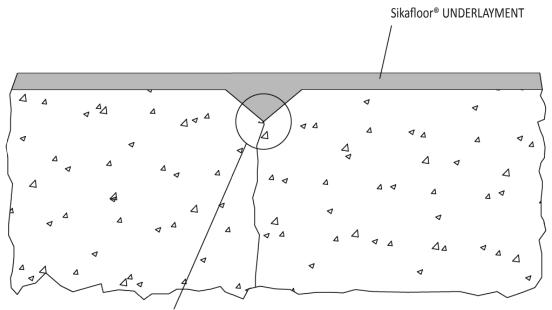
JOINT ROUTED OUT AND PRE-FILLED WITH MORTAR
