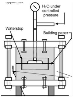
Based on test results for fluid migration, the U.S. Army Corps of Engineers recommends use of the conservative guidelines below for waterstop size selection.
