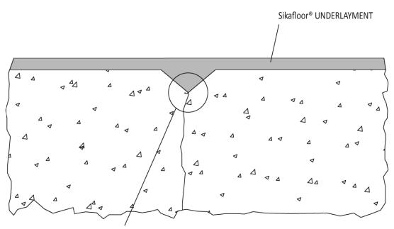
JOINT ROUTED OUT AND PRE-FILLED WITH MORTAR
