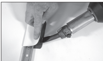
Welding protection pad
