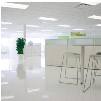
Once the old flooring material was completely removed and the concrete substrate carefully prepared and cleaned, a first coat of white-tinted Sikafloor® 261<sup>CA</sup> was applied. When dried, a second coat was applied to achieve a coating thickness of between 20 and 30 mils. Lastly, a coat of Sikafloor® Polythane UV® was applied to protect the floor against the yellowing effects of UV light, accentuate the glossy finish and render the floor chemical- and abrasion-resistant.
