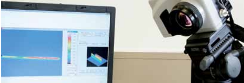
Sika's Systems Engineering supports the optimization of the adhesive application by patented test methods. Above image shows an infrared camera measuring the adhesive's reaction temperature.
