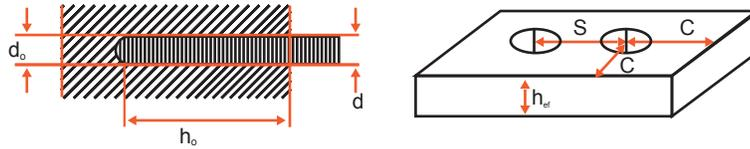
$h_{ef}$  = Effective anchorage depth (mm)
