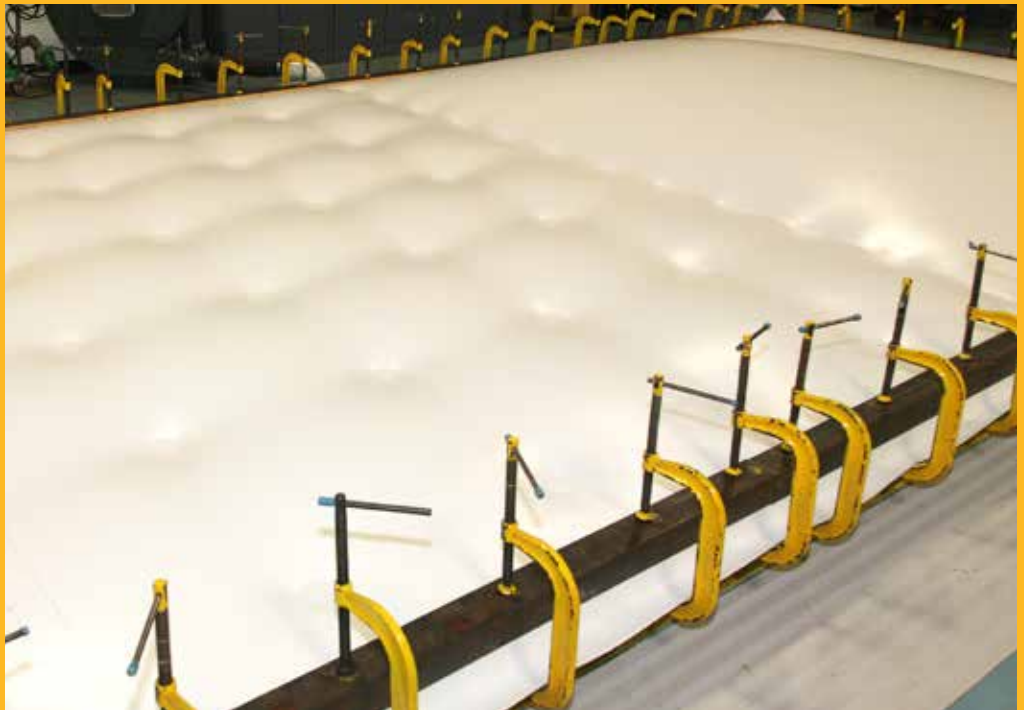
A PVC membrane undergoing wind resistance tests. The membrane is seen secured on the left portion of the test bed with the RhinoBond® tool, and at right using conventional in-seam attachment.
