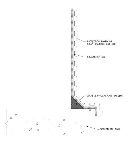
\*DRAINAGE MAT MAY BE TEMPORARILY HELD IN PLACE BY SIKAFLEX OR TWO-SIDED TAPE.
