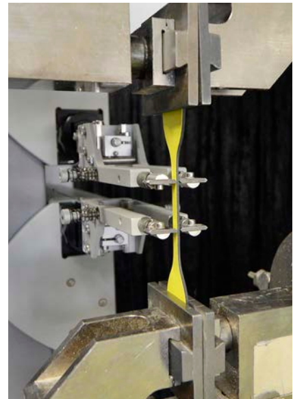
Determination of elongation and tensile strength of Sikaplan® PVC membrane after storage in hot water.
