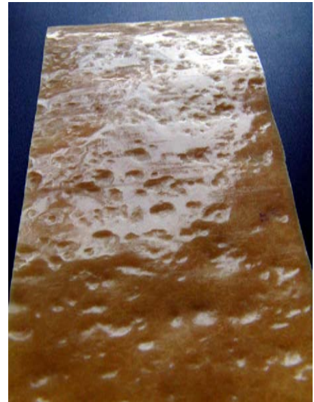
Membrane sample from excavated niche of the Reussport tunnel in Switzerland.
